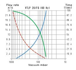
To calculate the emptying time of a volume of  $V_1$ , use the following formula:  $t_1 = \frac{t \times V_1}{100}$
