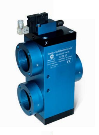
They are three-way vacuum solenoid valves, pilot-operated for capacities exceeding even 200 mc/h: They are used for vacuum interception on power supply units and suction palletizers, vacuum thermoformers, vacuum packaging units, robots, feeders, bag opening units and in all those cases where rapid exchange between pump suction for vacuums and air supply into the circuit is necessary for quick restoration of atmospheric pressure.
